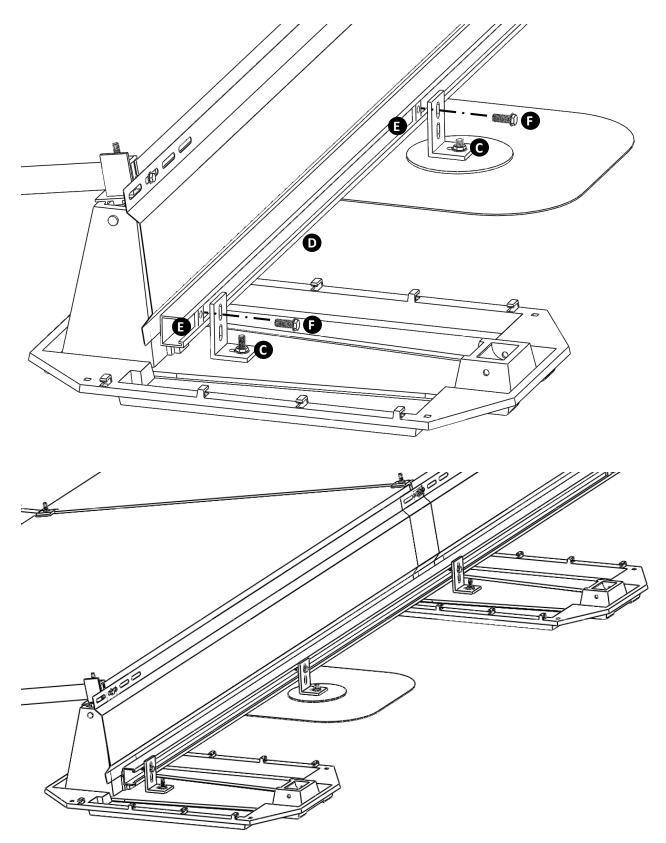
4. Attach Strut (D) to L Bracket using Bolt (F) and Strut Nut (E). Torque all Bolts (F) and Nuts (C) to 12 ft-lbs.
