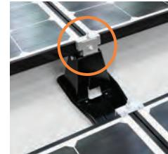
Space modules using alignment marks on Clamps, torque Nut provided to 14 ft-lbs.
