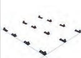
Measure & mark 2 chalk lines, Bases self-align as modules drop into place.
